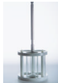
"B" Basket, (Test "B" 2.9.1.2 EP) 33 mm diam., used to test bigger samples order no. 105-2014 incl. glass tubes and disks
